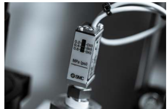
Pressure Switch to Monitor Incoming Air Supply for PLC Control Versions
