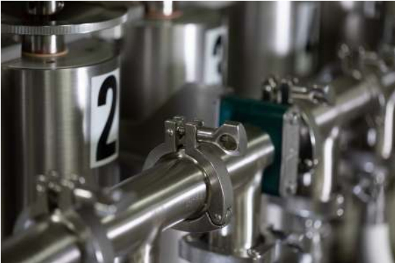
Easy Tri-clamp Breakdown for Cleaning or Change-over
